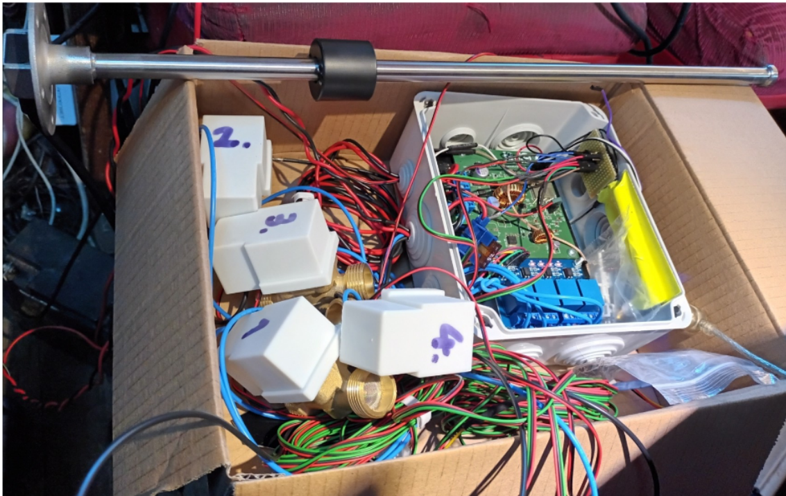
Figure 6: The electric/electronic part of irrigation computer system before installation. The tank fluid gauge sensor can be seen at the top (black ring = float).
