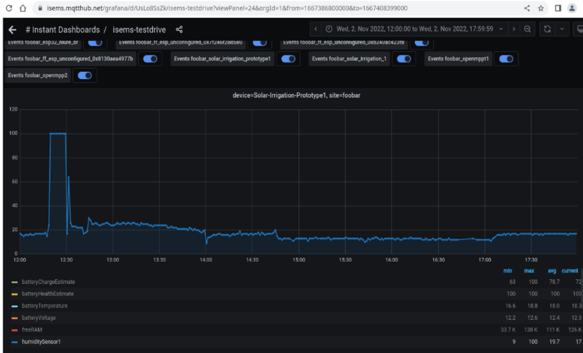
Figure 9: Humidity Sensor 1 data graph, recorded during lab testing.
