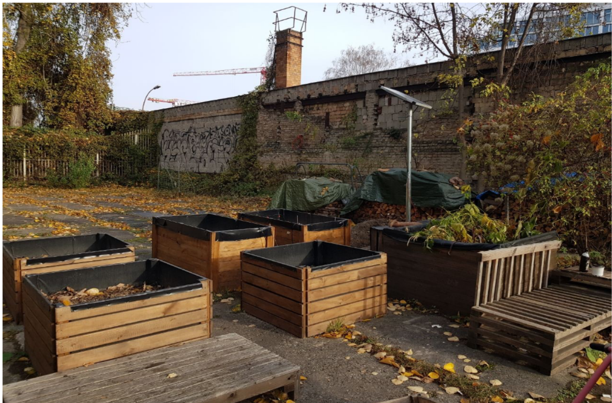
Figure 1: The prototype installation in winter with 6 plant beds. The 40 Watt solar module is mounted to a sturdy pole.
