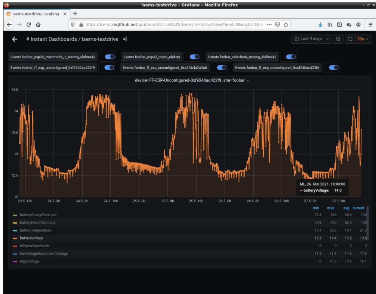
Mqttthub.net showing the battery voltage graph over the last 96 hours.
