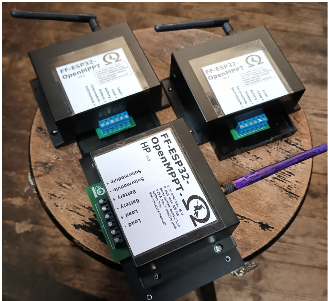
Figure 1: Two 100 Watt OpenMPPTs (top) and one 400 Watt OpenMPPT-HP
